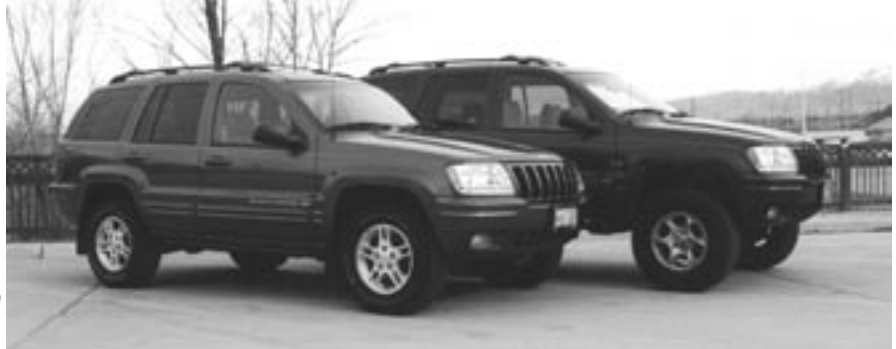
This photograph shows the difference between a stock WJ Grand Cherokee and a WJ Grand Cherokee with the four-inch suspension system (S4W).
